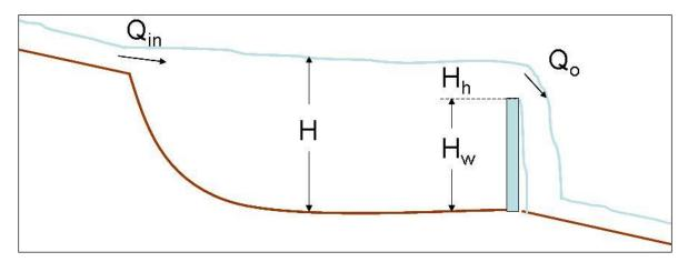
Figure 3 - Definition sketch for ponded flow
